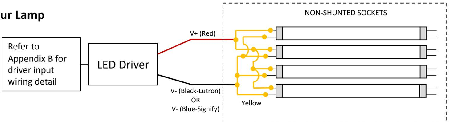
Illustration depicts existing luminaire wires and is for reference only. Your luminaire wire color, connection type and quantity may vary. INDIVIDUALLY CAP UNUSED WIRES.
