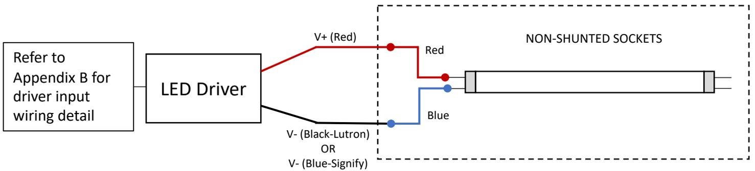
Illustration depicts existing luminaire wires and is for reference only. Your luminaire wire color, connection type and quantity may vary. INDIVIDUALLY CAP UNUSED WIRES.
