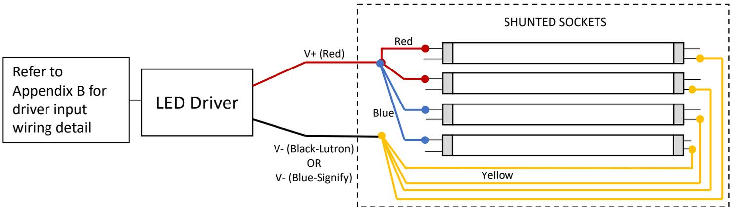
Illustration depicts existing luminaire wires and is for reference only. Your luminaire wire color, connection type and quantity may vary. INDIVIDUALLY CAP UNUSED WIRES.
