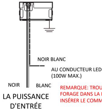
REMARQUE: TROU 25.4mm DE DIAMÈTRE DE FORAGE DANS LA PLAQUE DE MONTAGE POUR INSÉRER LE COMMUTATEUR D'ESSAI
