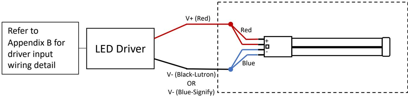
Illustration depicts existing luminaire wires and is for reference only. Your luminaire wire color, connection type and quantity may vary. INDIVIDUALLY CAP UNUSED WIRES.
