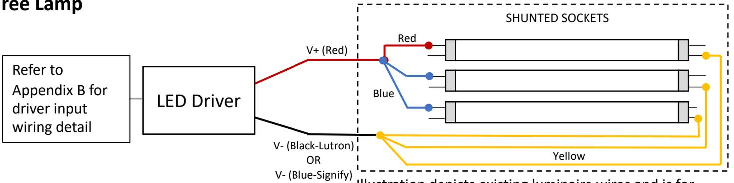
Illustration depicts existing luminaire wires and is for reference only. Your luminaire wire color, connection type and quantity may vary. INDIVIDUALLY CAP UNUSED WIRES.
